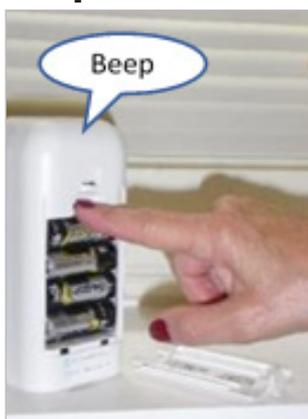
Remove the battery cover at the back of the AbiSensor.
