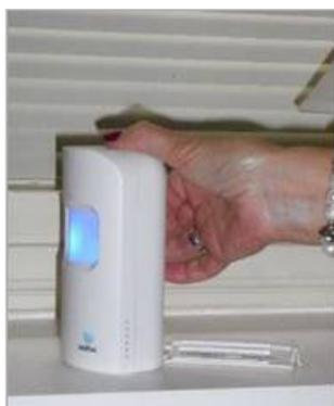
Once the AbiSensor is ON, press the **black button** again. The sensor will light up blue and enter Bluetooth mode.
